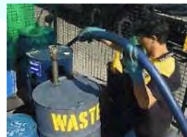
9. Clear labels and safe storage are required. Ensure spills cannot run outside the area.
