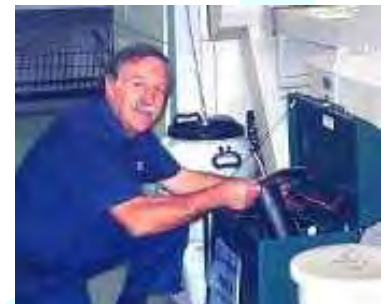
6.2 Servicing a SRU and harvesting the silver
